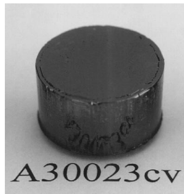
Figure 1.1: 1 inch diameter SiC boule grown at the IKZ, Berlin.
