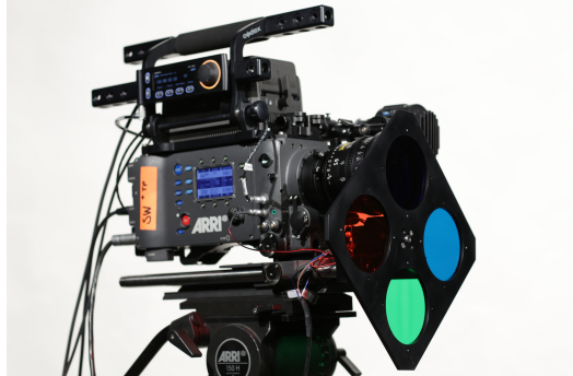
Figure 2.16: ARRI Alexa provided with a colour wheel. The picture was taken from [3].
