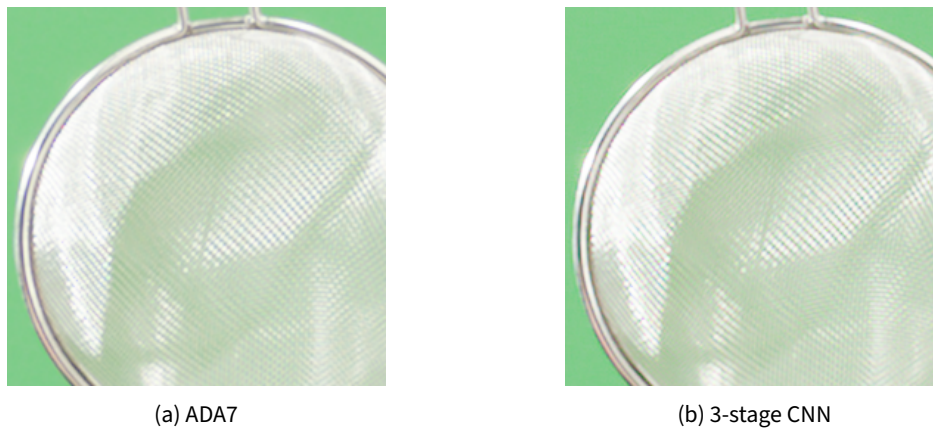
Figure 2.13: Evaluation of ADA7 and the 3-stage CNN on an image showing a sieve in front of a green screen. As can be seen, the 3-stage architecture shows some faulty colours in the high frequency areas and some staircase effects on the edges.
